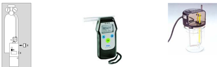
Fig. 2: dry-gas and wet-gas calibration equipment for breathalizers
