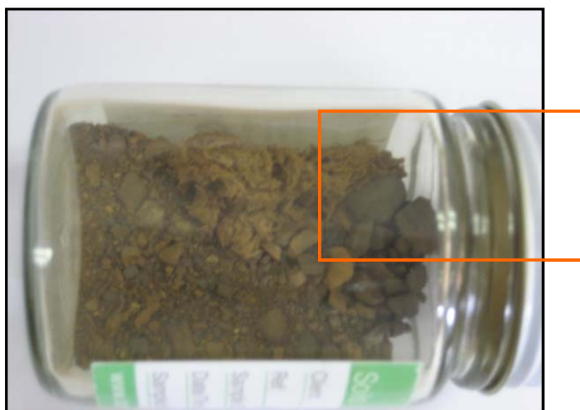
Figure 5: Spiked Sample 0.4 % Chrysotile, exhibiting non-homogeneity of fibres in the sample
