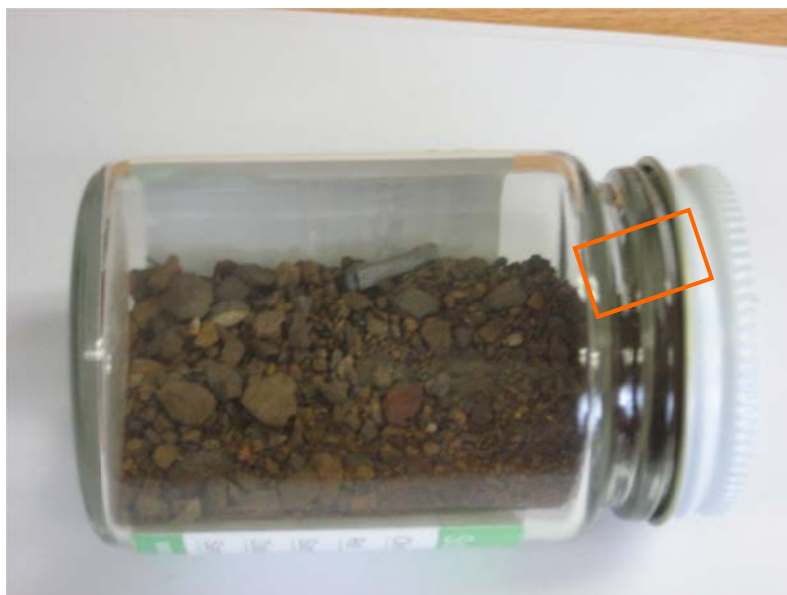
Figure 6: Spiked Sample 0.7 % Crocidolite, exhibiting non-homogeneity of fibres in the sample
