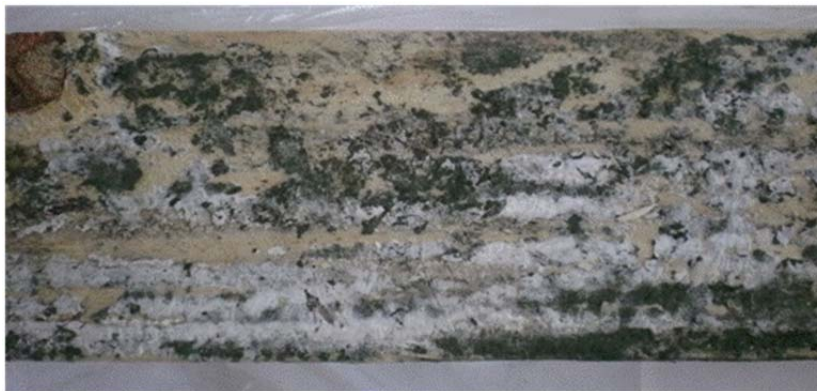
Figure 2: Contaminated timber handled by workers at Factory B
