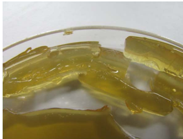
Figure 1: Damage to media plates when sampling at 100 l/min
