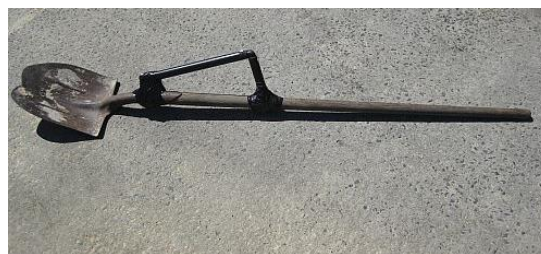
Figure 7. Supplementary handle design for shovel
