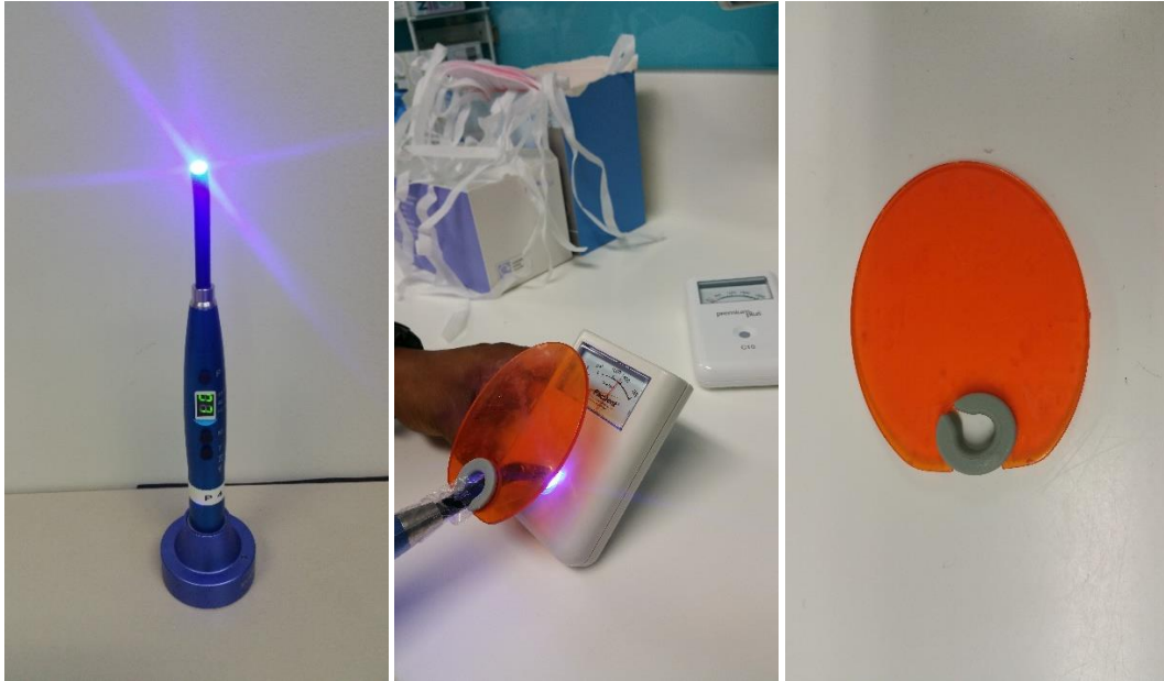
Figure 1. A dental curing lamp, digital radiometers and blue protective shield used in the dental simulation clinic.
