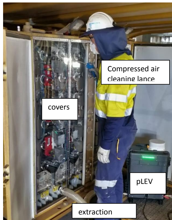
Figure 7 – Komatsu 960E electrical cabinet pLEV application. Note there is no visible dust.
