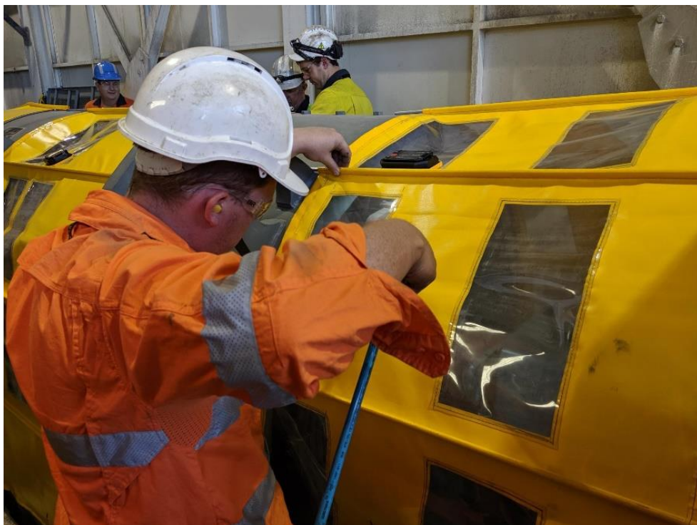
Figure 9 – MG set pLEV application. Note there is no visible dust.
