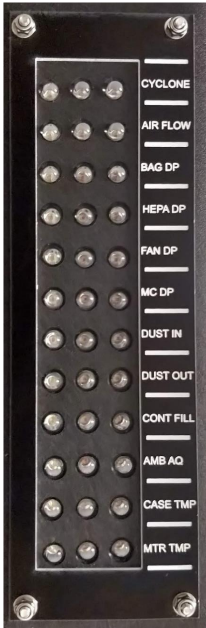
Figure 11 – Alarm display (LHS) and alarm description (RHS)
